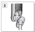
Fully insert the Stand Bracket into the speaker's clasp to stand speaker.
